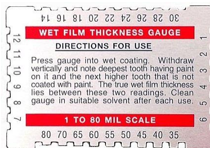
FIGURE 6 – Wet film thickness gauge.
